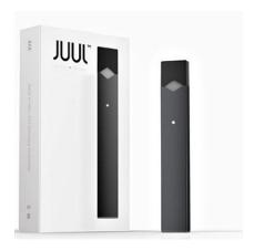
3. The user loads a "JUULpod," filled with a flavored liquid containing nicotine and other chemicals, into the JUUL vaping device. Powered by a battery that is charged through a USB port, the JUUL vaping device heats the liquid, converting the liquid into a vapor that the user breathes in through the mouth like someone smoking a cigarette.
